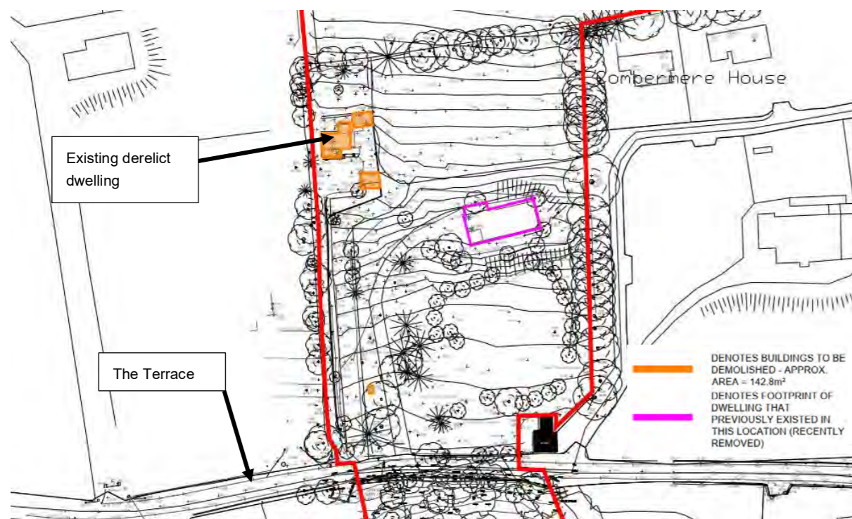
Figure 5 – Location of existing dwellings to be demolished
