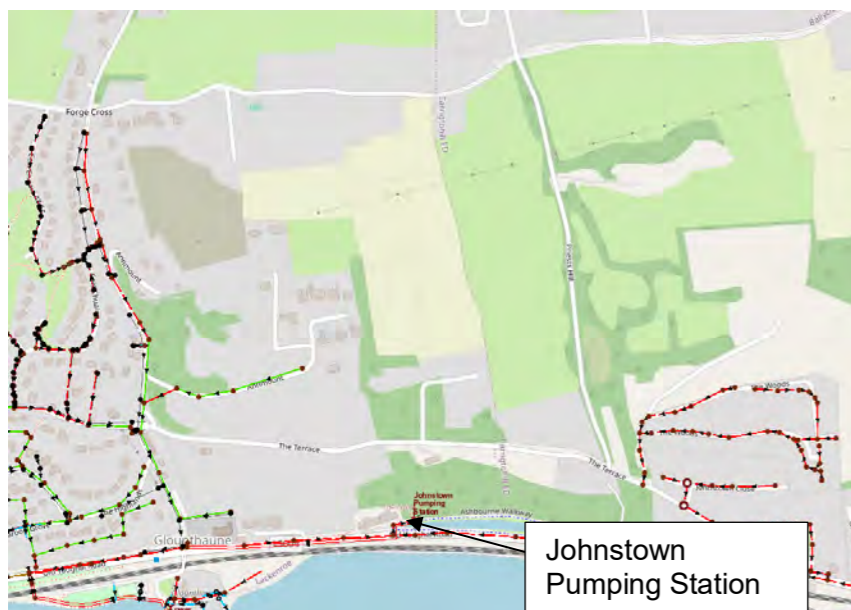
Figure 3-2 – Existing Wastewater Drainage Network
